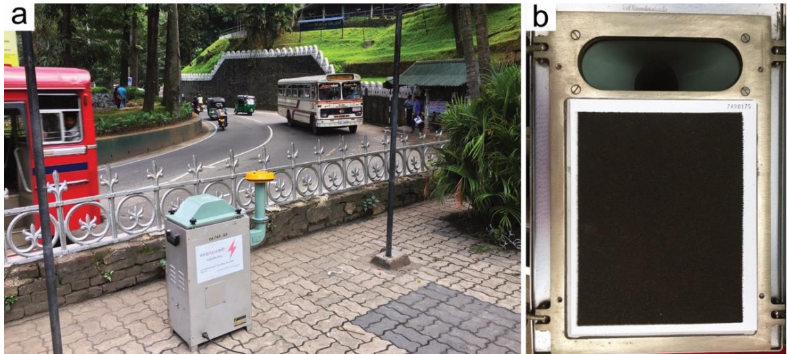
Fig. 4.1. Ambient air sample collection using high-volume respirable dust sampler operated at a constant flow rate of \sim 1.2 m 3 /min with glass microfiber filter paper. (a) Air sampler located
